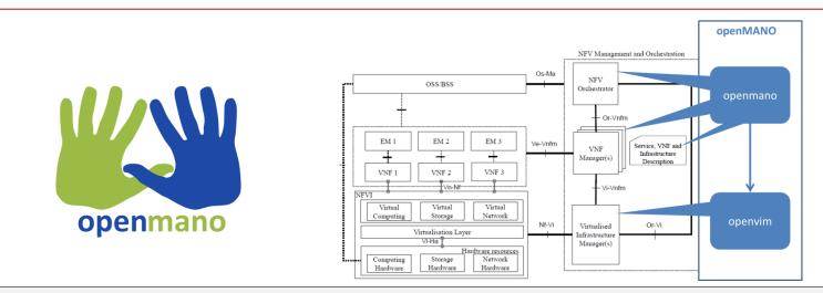
OpenMANO follows an NFVO-centric approach, granting the deterministic allocation of resources and with a simplified VNF instance lifecycle management at the NFVO (VNF instantiation and termination)
